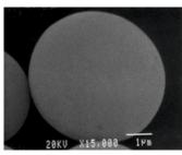
The pictures show the uniformity of the particle sizes and smoothness of particle surface, which enables more uniform packing with less channeling effect. This leads to lower back pressure and the higher column efficiency. Our silica has a surface area of  $320 \text{ m}^2/\text{g}$  with a controlled mean pore size of 120 Å.
