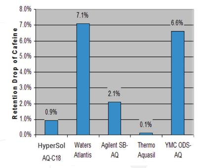
Under the same condition, when compared with other AQ-C18 columns at highly aqueous mobile phase, HyperSol AQ-C18 shows excellent resistant to phase collapse.
